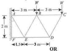
Explain the procedure to find forces in members of truss by using CO5 L2 10M method of joints.
